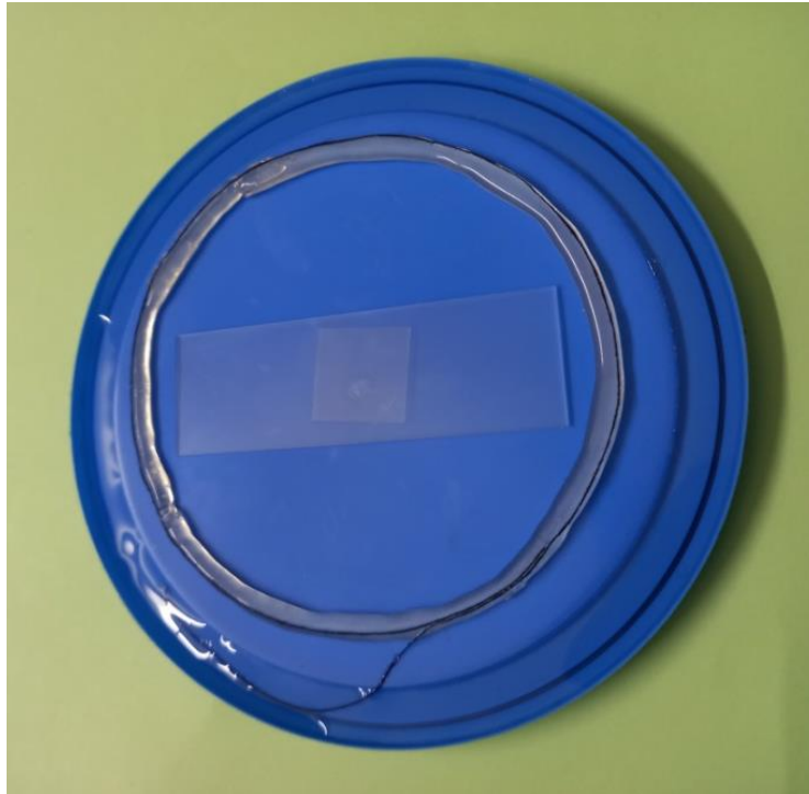
Fig. 2. The design based on placing the diet between two glass slides
