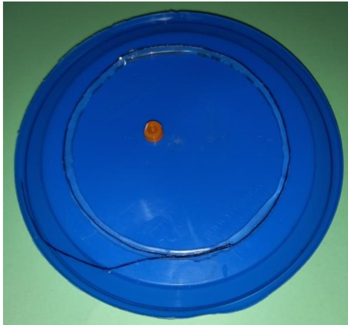
Fig. 4. The design based on placing a drop of the diet in a tiny plastic pot
