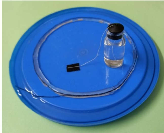
Fig. 6. The design based on placing a drop of the diet on a piece of cloth connected to a water-saturated thread
