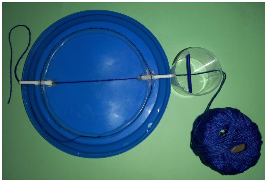
Fig. 3. The design based on presenting a drop of the diet via a thread connected to a little of the diet
